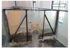
Figure 4a: Water-sediment mixture outflow during Run no. 1
