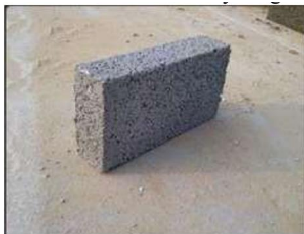
Figure 2: Recycled cement bricks, from construction debris, sand and gravel
