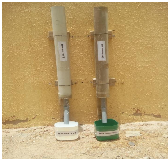
Figure 4: Experimental pilot of sand filtration
