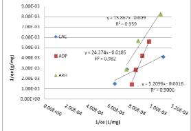
Fig. 7. Langmuir isotherm for COD reduction in resin wastewater onto CAC, ADP and ARH.
