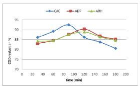
Fig. 3. The effect of varying the stirring/ contact time (min) upon %COD reduction at pH 7, adsorbent weights (30 g/L CAC, 40 g/L ADP and 60 g/L ARH),  $T=25^{\circ}C$ , volume of solution 50 mL, and  $COD_{o}=8210$  mg/L.
