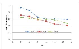
Fig. 4. The effect of varying pH upon %COD reduction, adsorbent weights (30 g/L AC, 40 g/L ADP and 60 g/L ARH),  $T=25^{\circ}C$ , volume of solution 50 mL, and  $COD_{o}=8210$ mg/L.
