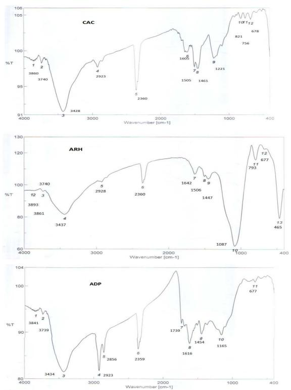
Fig 1. FTIR spectra of commercial activated carbon (CAC) and prepared activated date pits (ADP) and activated rice husks (ARH).
