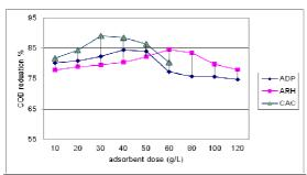
Fig. 2. The effect of adsorbent weight (ADP, ARH and CAC) upon COD reduction % at pH 7;  $t_{CAC}$ = 90 min,  $t_{ADP}$  =120 min and  $t_{ARH}$ = 120 min; T= 25°C, volume of solution 50 mL, and COD $_{o}$  = 8210 mg/L.
