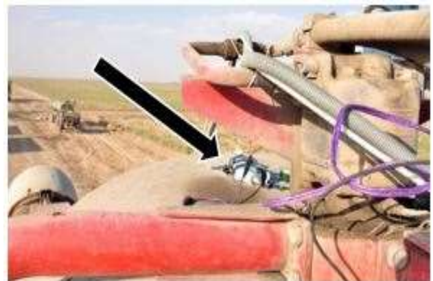
Figure.3: The windshield used and how to place the microphone inside it
