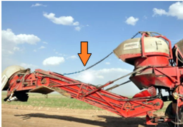
Figure 4: Cabling toward driver's cabin
