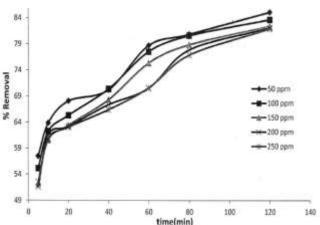
Figure 8: Effect of % removal and contact time on the adsorption of different initial concentrations
