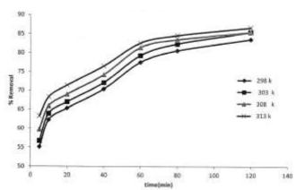
Figure 12: Effect of time on % removal of Cd2+ and different temperatures
