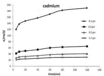
Figure 10: Effect of adsorbent dose on the removal of  $Cd^{2+}$  and  $q_e$  on the adsorption of different doses of guava leaves
