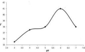
Figure 3: Effect of pH on adsorption of Cd2+
