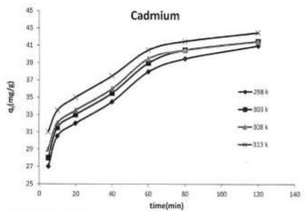
Figure 13: Effect of time on  $q_t(mg/g)$  of  $Cd^{2_+} adsorption$  and different temperatures
