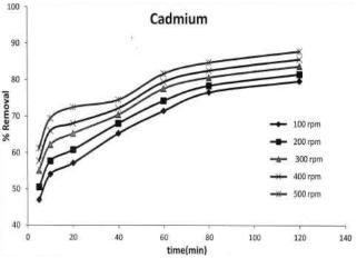
Figure 11: Effect of contact time on the adsorption of Cd<sup>2+</sup> at different rpm
