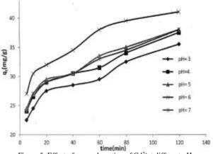
Figure 5: Effect of q<sub>t</sub> on adsorption of Cd<sup>2+</sup>at different pH
