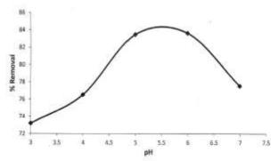
Figure 4: Effect of pH versus Cd<sup>2+</sup> removal percentage
