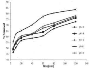
Figure 6 % removal of Cd2+ at different pH
