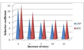
Figure 6: Comparison of behavior coefficient of two-span structures designed with stud brace sections and can brace sections under triangular loading pattern.
