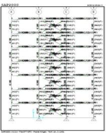
Figure 2: Assign of plastic joint
