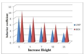
Figure 5: Comparison of behavior coefficient of three-span structures designed with stud brace sections and can brace sections under triangular loading pattern.
