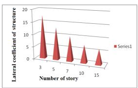
Figure 4: Lateral capacity diagram for three-span structures designed with stud brace sections under triangular loading pattern.
