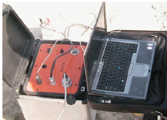
Fig (1-24): The used seismograph, ABEM RAS 24 apparatus
