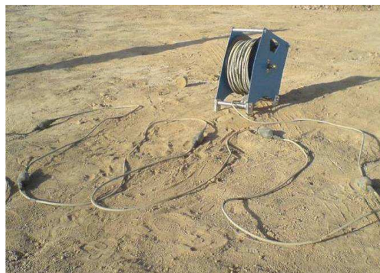
Fig (1-27): A picture of the used geophones in seismic tests
