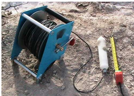
Fig (1-28): A picture of the used down hole geophones
