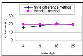
Figure 5: Critical load for increasing of plate grids
