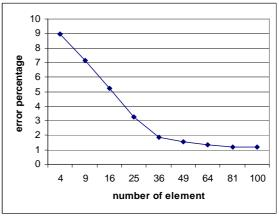
Figure 8: Error changes for different plate elements
