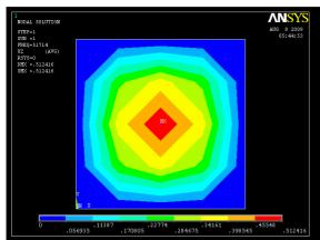
Figure 10: deformation model of plate in ANSYS software
