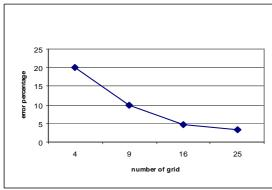
Figure 6: Error changes for increasing of plate grids
