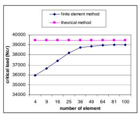
Figure 7: Critical load of plate for different number of elements
