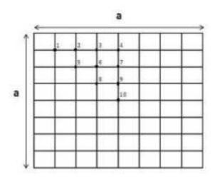
Figure 4: grids of plate in finite difference method
