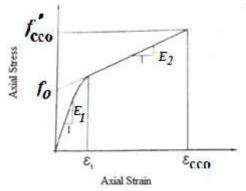
Figure 2: Changes of the confined concrete stress - strain in lam model.
