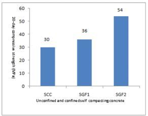
Figure 8: Compressive strength of SCC, SGF1 and SGF2
