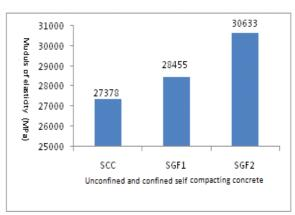
Figure 12: Modulus of elasticity of SCC,SGF1 and AGF2
