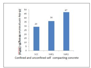
Figure 7: Compressive strength of SCC, SGF1 and SGF2
