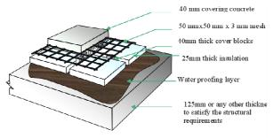
Figure 4: Detailed arrangement of the insulation system proposed over reinforced concrete slabs
