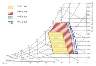
Figure 3: Modified comfort zone when the out door temperature increase by  $4^{\,0}\text{C}$
