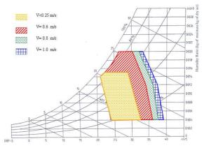
Figure 2: Modified comfort zone when the outdoor temperature increase by  $2\,^{0}\mathrm{C}$
