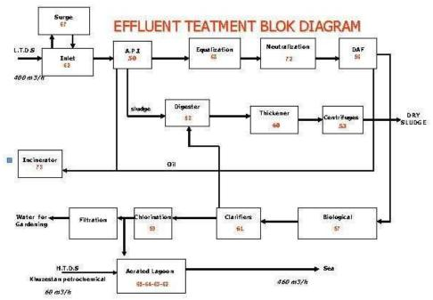
Figure 2: Wastewater treatment process diagram
