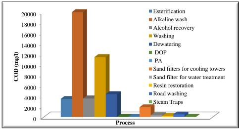
Figure 3: comparing of effluent COD in different processes
