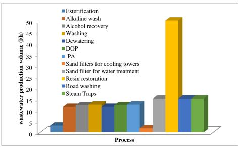
Figure 4: comparing of wastewater production volume (liters per hour) in the effluent of processes
