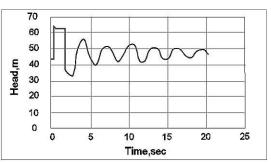
Figure 2: Pressure changes as compared to time according to research conducted by covas et al [10].
