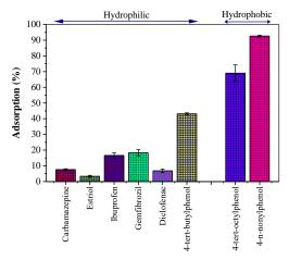
Figure 4: Adsorption of hydrophilic and hydrophobic TrOCs to the NF270 membrane at pH 11. The error bars present standard deviation of data obtained from two independent experiments
