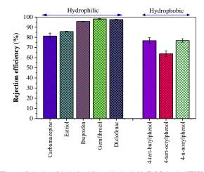
Figure 6: Rejection of the hydrophilic and hydrophobic TrOCs by the NF270 membrane at pH 7. The error bars present standard deviation of data obtained from two independent experiments
