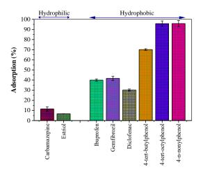
Figure 2: Adsorption of hydrophilic and hydrophobic TrOCs to the NF270 membrane at pH 4.7. The error bars present standard deviation of data obtained from two independent experiments
