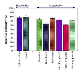
Figure 5: Rejection of the hydrophilic and hydrophobic TrOCs by the NF270 membrane at pH 4.7. The error bars present standard deviation of data obtained from two independent experiments
