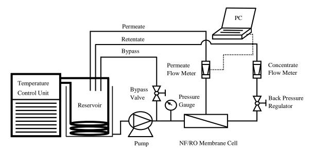
Figure 1: Schematic diagram of the cross flow NF/RO filtration system
