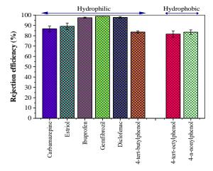
Figure 7: Rejection of the hydrophilic and hydrophobic TrOCs by the NF270 membrane at pH 11. The error bars present standard deviation of data obtained from two independent experiments
