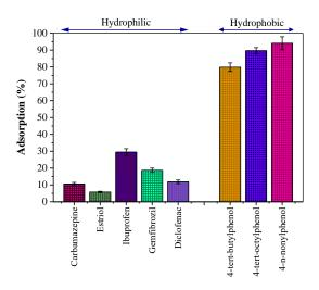
Figure 3: Adsorption of hydrophilic and hydrophobic TrOCs to the NF270 membrane at pH 7. The error bars present standard deviation of data obtained from two independent experiments
