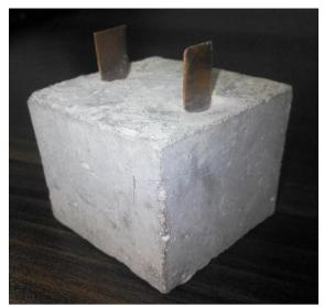
Fig 1: Specimen for resistivity measurements
