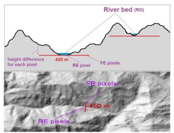
Figure 2: The schematic illustration of the FHD model; the upper is a schematic profile and the lower is a top view.
