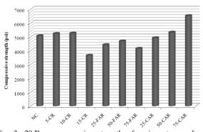
Fig. 3: 28-Days compressive strength of various types of concrete used in the study (NC = Normal concrete, 5,10,15-CR = Percentage cement replacement, 25,50,75-FAR/CAR = Percentage fine/coarse aggregate replacement)
