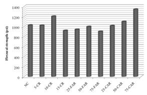
Fig. 4: 28-Days flexural strength of various types of concrete used in the study (NC = Normal concrete, 5,10,15-CR = Percentage cement replacement, 25,50,75-FAR/CAR = Percentage fine/coarse aggregate replacement)
