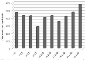
Fig. 2. 14-Days compressive strength of various types of concrete used in the study (NC = Normal concrete, 5,10,15-CR = Percentage cement replacement, 25,50,75-FAR/CAR = Percentage fine/coarse aggregate replacement)
