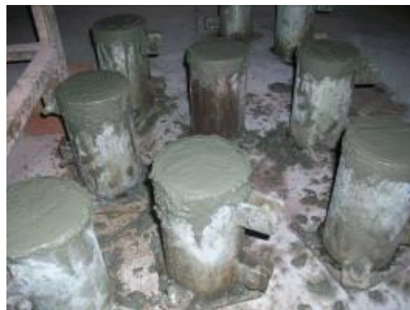
Figure 3: Preparing concrete cylinder
