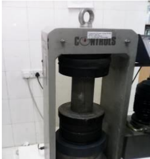
Figure 4: Compressive strength testing of concrete cylinder with universal testing machine (UTM)
