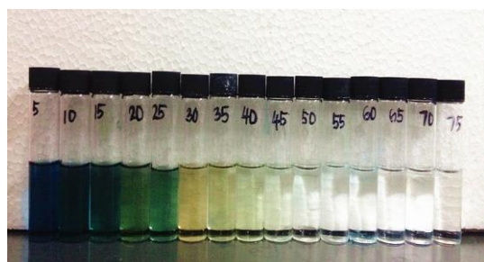
Figure 3: Change in colour of MB solution (100 ppm) by the oxidation of SPS (100 mM) with respect to different times showing complete decolourisation in 60 min. Experimental condition: pH ~ 7.0, Temperature = 70 °C.
