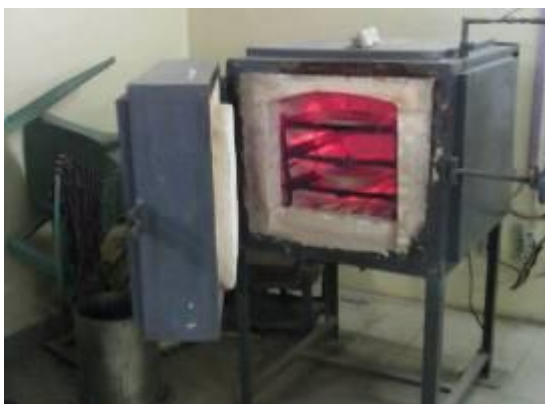
Figure 2: Sugarcane Bagasse burning in the oven at Lab
