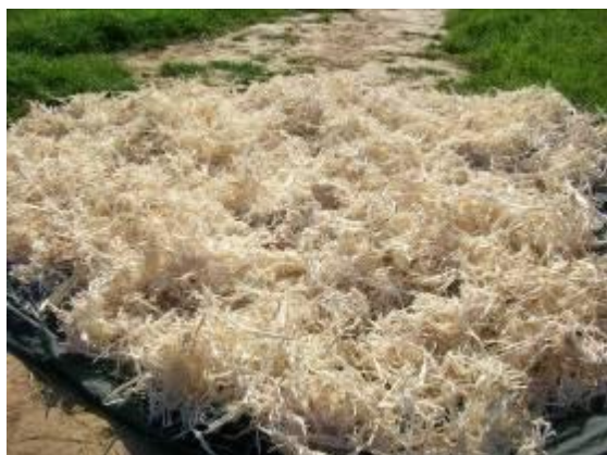
Figure 1: Sugarcane Bagasse was drying under the sun light after collecting from sugar mill
