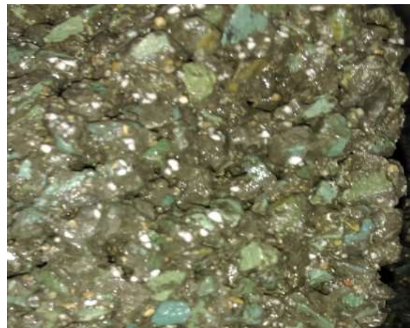
Figure 6: Section of porous concrete containing zeolite (above) and perlite (below)
