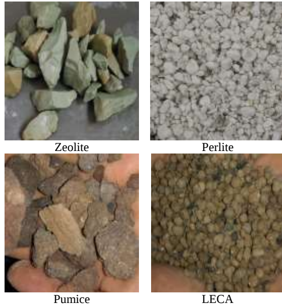
Figure 2: Applied additives in porous concrete mixture designs
