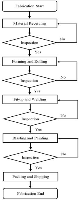
Figure 1: Fabrication of pressure vessel flowchart
