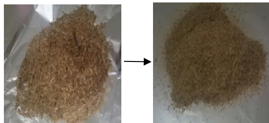
Figure 1: RH before and after grounding
