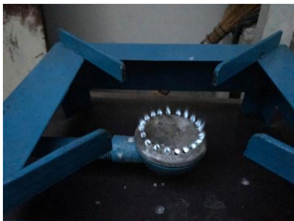
Figure 5: A blue flame indicating produced biogas had methane content
