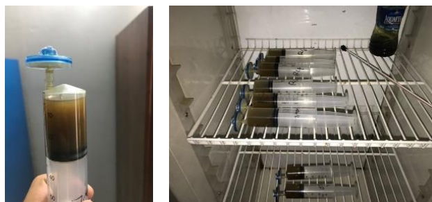
Figure 1: Syringe reactor used in the BMP study
