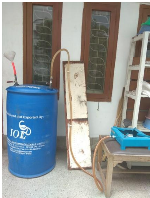
Figure 2: Field trial biogas reactor and burner
