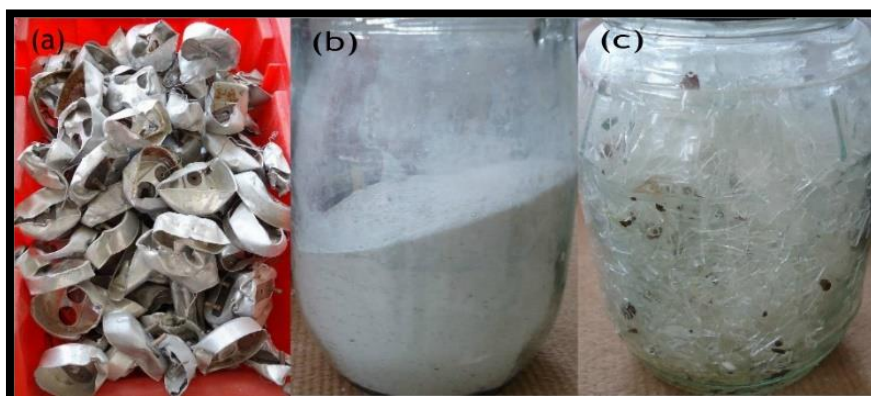
Figure 2: Output products of the lamp crusher: Separated aluminum (a), phosphor powder (b) and glass (c)
