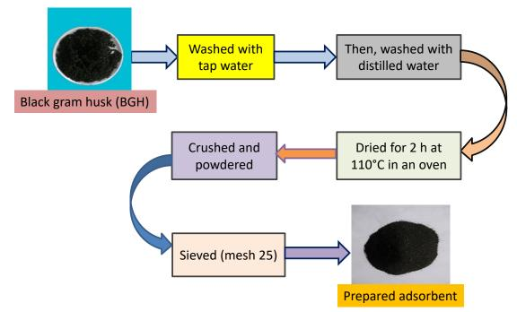
Figure 1: Flow diagram for the preparation of adsorbent
