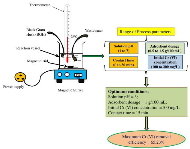
Figure 2: Experimental set-up with range of process parameters
