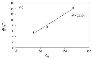
Figure 8: (a) Freundlich isotherm (b) Langmuir isotherm for the Cr (VI) adsorption on BGH (Experimental conditions: Adsorbent dosage = 1 g/100 mL; Solution pH = 3; T = 25°C; Time = 15 min; Solution volume = 100 mL)
