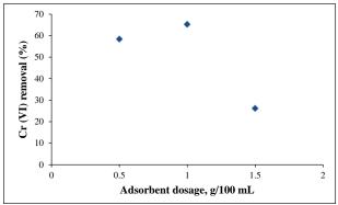
Figure 5: Effect of adsorbent dosage on the removal efficiency of Cr (VI) (Experimental conditions: Solution pH=3;  $T=25^{\circ}C$ ; Time = 15 min; Initial Cr (VI) concentration = 100 mg/L, Solution volume = 100 mL)
