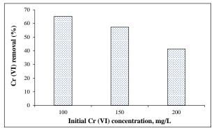
Figure 6: Effect of initial Cr (VI) concentration on the removal efficiency of Cr (VI) (Experimental conditions: Adsorbent dosage = 1 g/100 mL; Solution pH = 3; T =  $25^{\circ}$ C; Time = 15 min; Solution volume = 100 mL)
