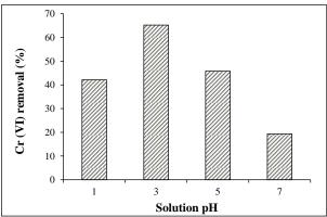
Figure 4: Effect of solution pH on the removal efficiency of Cr (VI) (Experimental conditions: Adsorbent dosage = 1 g/100 mL; T = 25°C; Time = 15 min; Initial Cr (VI) concentration = 100 mg/L, Solution volume = 100 mL)
