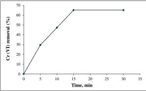
Figure 7: Effect of contact time on the removal efficiency of Cr (VI) (Experimental conditions: Adsorbent dosage = 1 g/100 mL; Solution pH = 3; T = 25°C; Initial Cr (VI) concentration = 100 mg/L; Solution volume = 100 mL)
