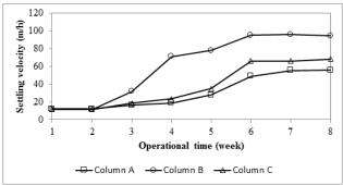
Figure 3: Settling velocity of activated sludge
