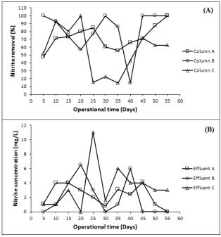
Figure 7: Profile of the nitrite removal performance (A) and concentration (B) in all columns
