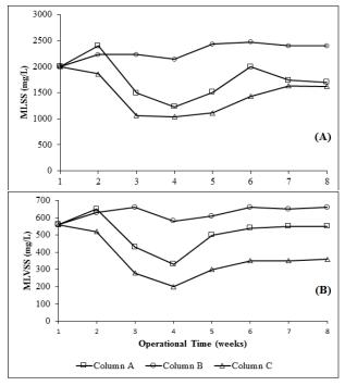
Figure 2: Profile of biomass concentration (A) MLSS (B) MLVSS in all columns
