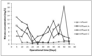
Figure 8: Influent-effluent nitrate concentration in Column A, Column B and Column C
