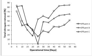
Figure 9: Removal performance of total nitrogen in all columns
