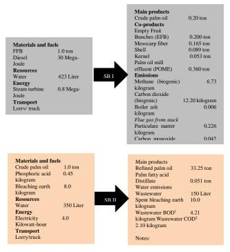
Figure 2: Inventory analysis of system boundary 1 (SB I) and system boundary 2 (SB II)
