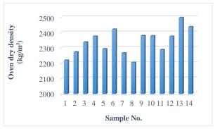
Figure 7: The results from oven dry density test, age 28 days
