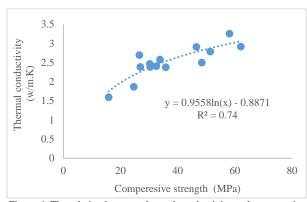
Figure 6: The relation between thermal conductivity and compressive strength of normal weight concrete
