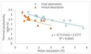
Figure 10: The relation between thermal conductivity and water absorption of normal weight concrete
