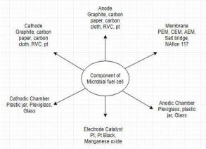
Figure 2: Components of microbial fuel cell
