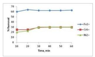
Figure 4: Effect of contact time on removal percentage of metal ions
