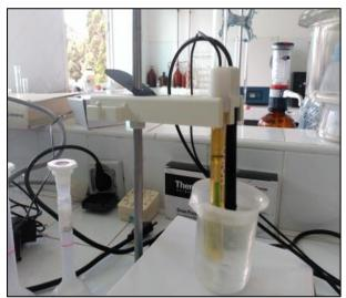
Figure 3: Measure of F- by the electrode specific
