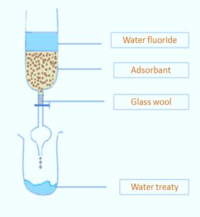
Figure 1: Elimination of fluorine by activated alumina / activated charcoal
