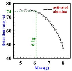
Figure 8: Retention rate % (activated alumina)
