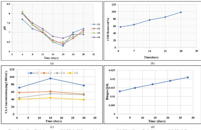
Figure 2: (a) pH profile during start-up of MABR (b) COD removal during start-up of MABR (c) VA profile during start-up of MABR (d) Biogas production during start-up MABR
