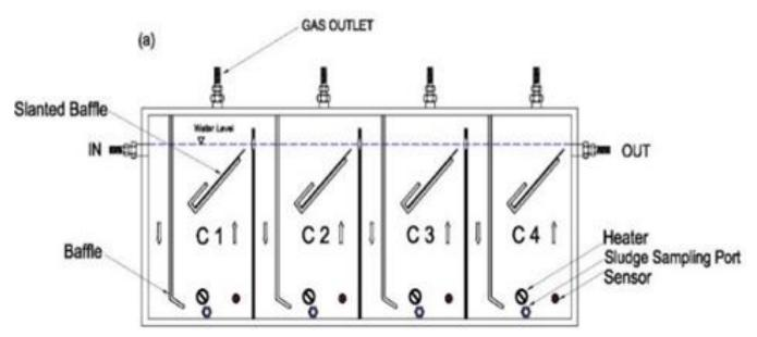
Figure 1: Schematic diagram showing modified anaerobic baffled reactor (MABR)
